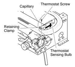
Figure 48 - Removing Thermostat Sensing Bulb
